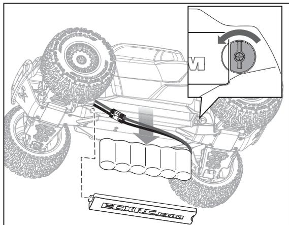
4. Disconnect the battery from the ESC/Receiver unit.
