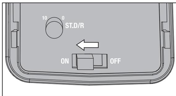
2. Connect the battery to the Electronic Speed Control (ESC) / Receiver unit and power on the vehicle.
