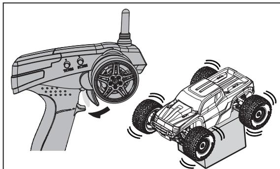
4. Start driving slowly. If the wheels are not straight, adjust the steering trim dial on the transmitter.
